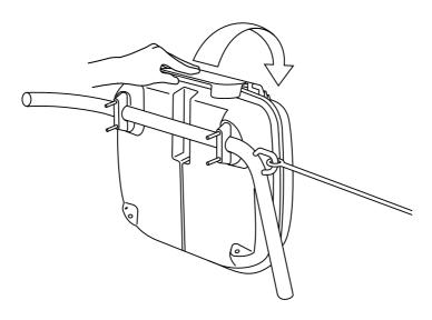
3.1.2 Upon release, the container will open and the recovery module will automatically fall outboard and automatically inflate.
