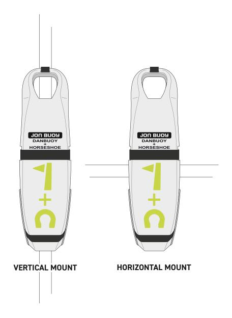
This leaflet details the installation and mounting instructions of the Danbuoy marker & Inflatable Horseshoe in either a vertical or horizontal orientation.
