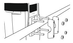
3. Tighten the Nyloc nuts until the bracket does not rotate on the bar when pushed.
